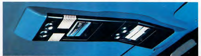
Roof storage console with dome and reading lamps
