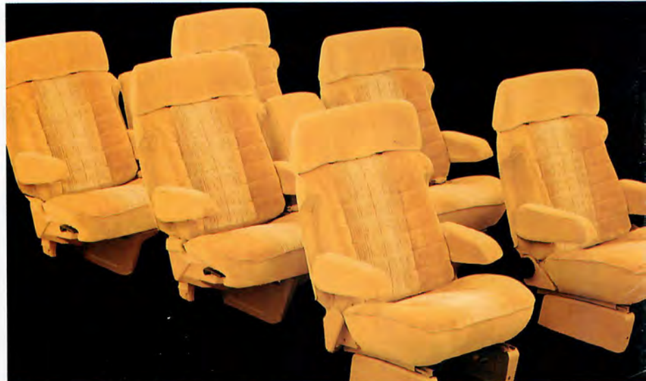
SLT interior with available 8-person seating arrangement (rear seat center backrests shown folded down)
