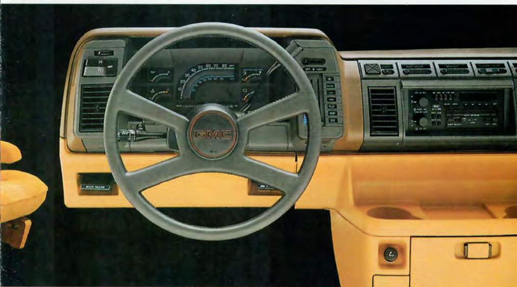
New, restyled instrument panel for all models has larger glove box and improved air distribution. Gage-type instrumentation is standard.
